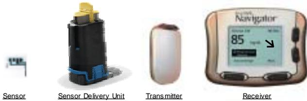
The FreeStyle Navigator Continuous Glucose Monitoring System measures interstitial fluid glucose every minute using a patient-inserted electrochemical sensor. The system was developed by Abbott Diabetes Care and is currently available for Investigational Use Only.
